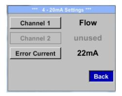
To make changes, first select a menu with button  $^{"}_{"}\Delta"$  and confirm selection by pressing  $^{"}_{"}OK"$ .
