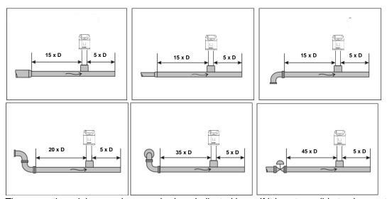
The respective minimum values required are indicated here. If it is not possible to observe the stipulated equalising sections, considerable deviations in the measuring results must be expected.
