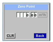
When, without flow, the installed sensor shows already a flow value of > 0 m<sup>3</sup>/h herewith the zero point of the characteristic could be reset.
