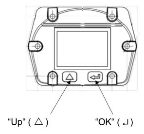
The operation of the VA 520 is done by the two capacitive key buttons Up ( $\triangle$ ) and Enter ( $\checkmark$ )
