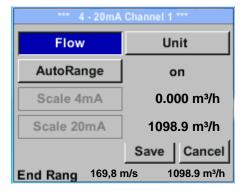
The 4-20 mA Analogue output of the Sensor VA 520 can be individually adjusted.
