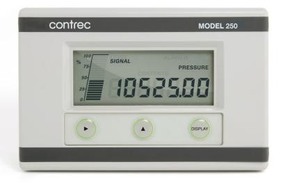
The 250 Programmable Process Indicator accepts a 4-20mA signal from a wide range of transducers such as pressure or temperature transmitters, weigh scales, pH sensors, flowmeters or level transmitters. The Indicator will display the signal level on the bar graph and the scaled process variable on the large numeric display.
