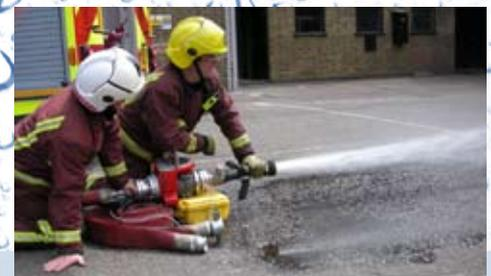
Using the Flowmaster to test fire fighting equipment
