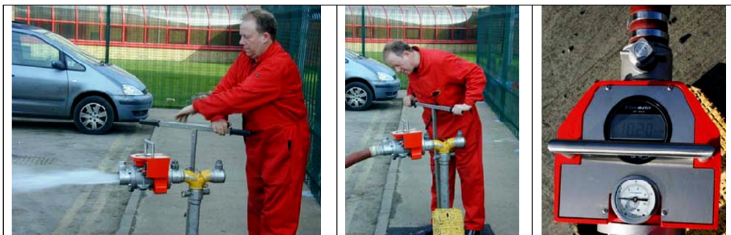
Figure 7: Testing an underground hydrant using a standpipe and an example of flow readout and residual pressure reading. Photos courtesy of Essex County Fire and Rescue Service and Laois Fire Service.
