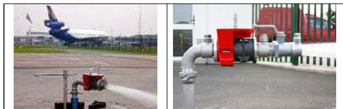
Figure 8: Flow testing at Manchester Airport with no attachment to outlet and flow testing with a ball valve to facilitate static and residual pressure measurements at Portlaoise Hospital. Photos courtesy of Manchester Airport and Portlaoise Hospital Service respectively
