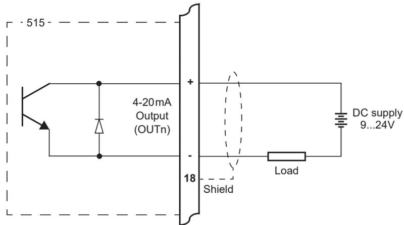
Figure 12 Output 4-20mA Connection Diagram
