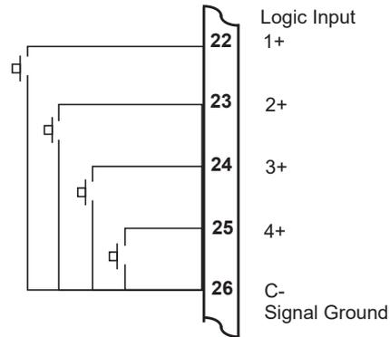
*Figure 11 Logic Inputs Connection Diagram*
