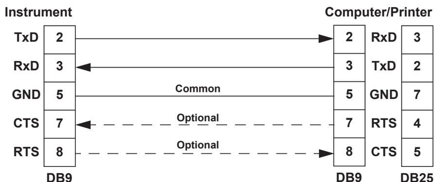
Figure 19 RS-232 Cable Connections to a Computer
